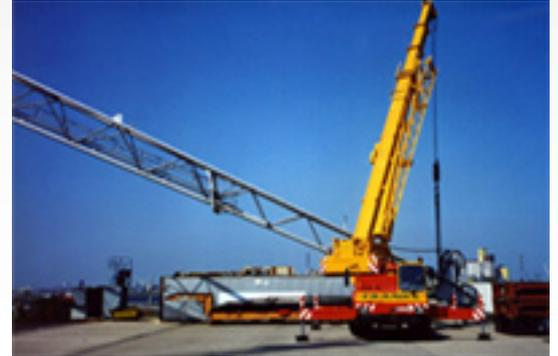
16ton MAN Travelling gantry Crane - Boom being assembled
